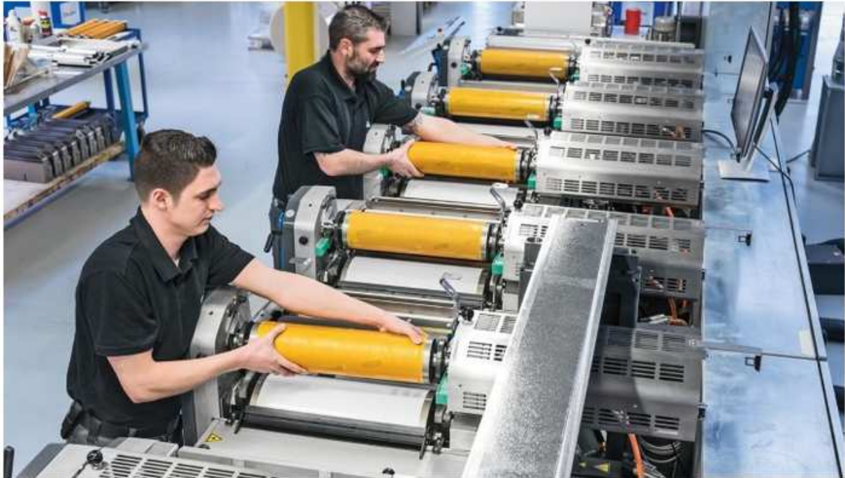
Exceptionally short set-up times and superfast job changes due to the gearless lightweight printing cylinders. (Photo: Gallus Ferd. Rüsch AG)
