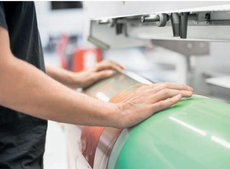
Left: Plate mounting on a Twinlock Sleeve.
