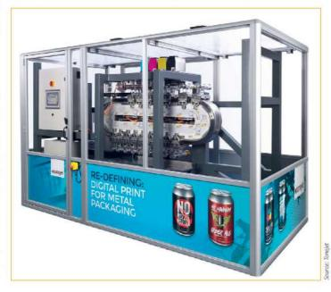
The iTrak transport system positions the cans exactly under the print heads
